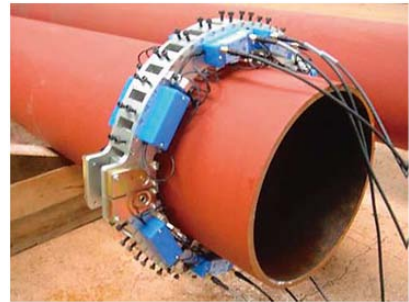
Figure 3.11 A guided wave sensor that can perform wall thinning inspection of piping [Odakura. 2009].
