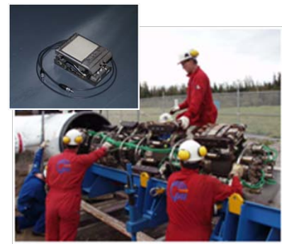
Figure 3.9 Prototype EmatScan CD pig for inspection of pipelines. Also shown (top corner) is the SH-wave probe in a spring loaded suspension [Salzburger. 2009].
