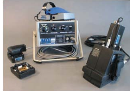
Figure 3.1 Industrial MOI system for inspection of aging aircrafts. [Shih et al ]
