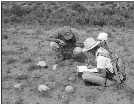
*The vegetative cover is documented at a test plot on a reclaimed haul road near the Gunnison, Colorado, Disposal Site.*
