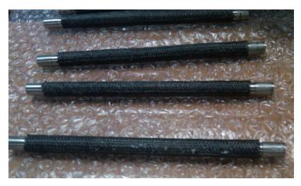
Figure 13. Silicon carbide clad test rodlets.
