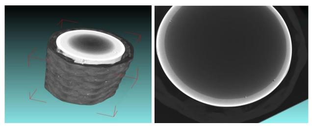
Figure 15. Micro-tomographic image of silicon carbide ceramic matrix composite test rodlet, showing the zirconium liner and silicon carbide ceramic matrix composite.
