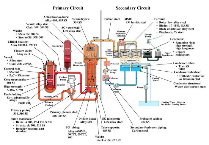
Figure 7. Sampling of the typical materials in a pressurized water reactor.
