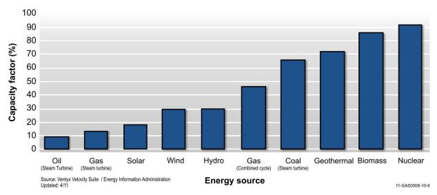
Figure 2. United States electrical generation capacity factors by energy source, showing high operating performance.
