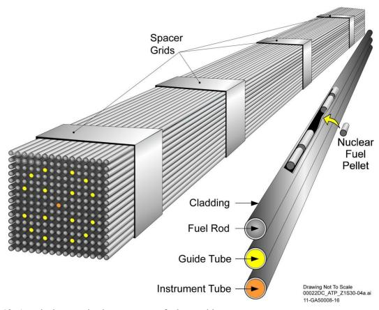
Figure 12. A typical pressurized water reactor fuel assembly.
