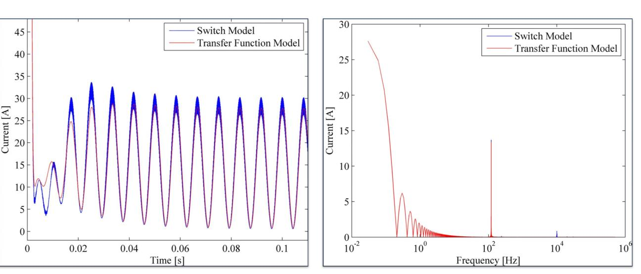
Time domain and frequency domain simulation results are shown for the switch level model vs. the proposed model with an ideal 60 Hz input (Left).
