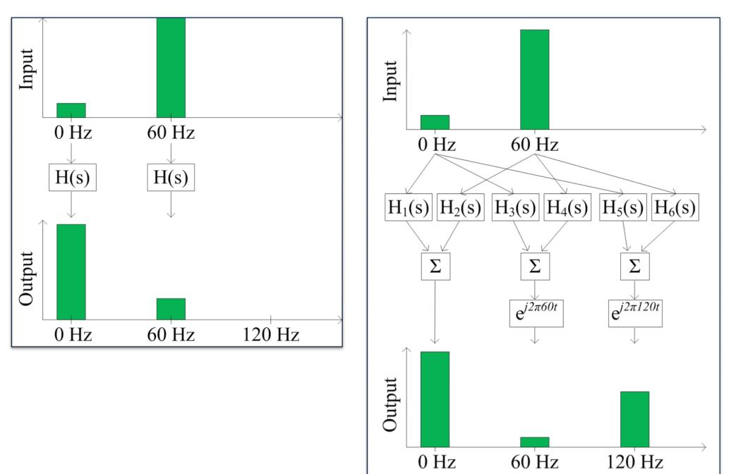
Standard transfer functions (left) can only map each frequency onto itself. As a result, any nonlinear relationships in a system are lost. Using standard TF's to analyze a battery's frequency content yields inaccurate results. Harmonic transfer functions (right) preserve nonlinear relationships and allow the system to be modeled in a linear fashion. The system can then be analyzed using well established techniques.
