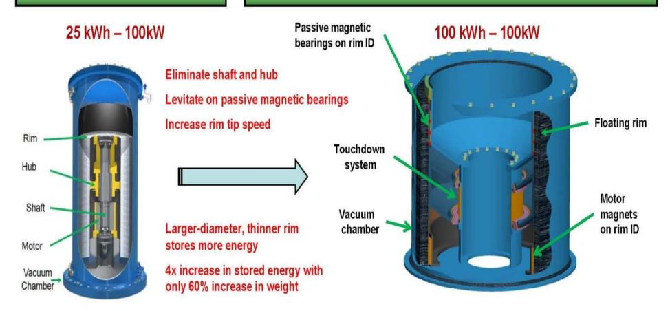
Program Tasks – Develop Bonded Magnets, Touchdown Bearings, and Low Cost Rim
