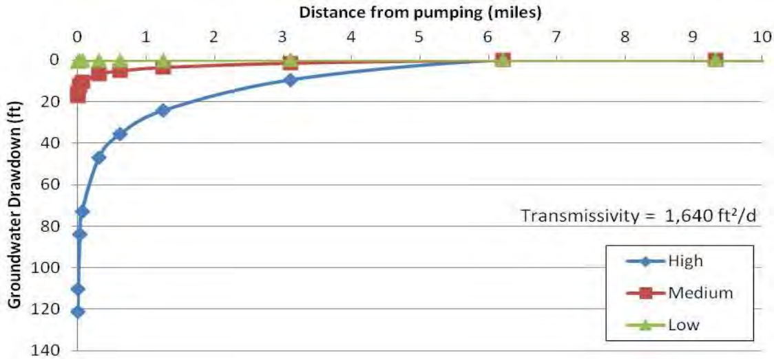
FIGURE 11.3.9.2-2 Estimated One-Dimensional Groundwater Drawdown Resulting from High, Medium, and Low Groundwater Pumping Scenarios over the 20-Year Operational Period at the Proposed Dry Lake SEZ as Revised
