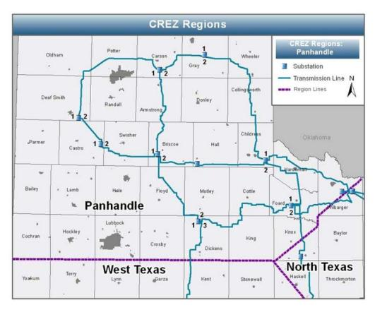
Figure 3-2. Transmission Lines and Substations Proposed for the Texas Panhandle Region (Source: PUCT 2012b, all)
