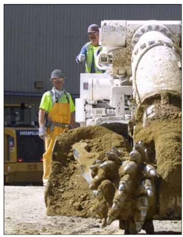
Figure 2-5 Road Header Used for Tunneling
