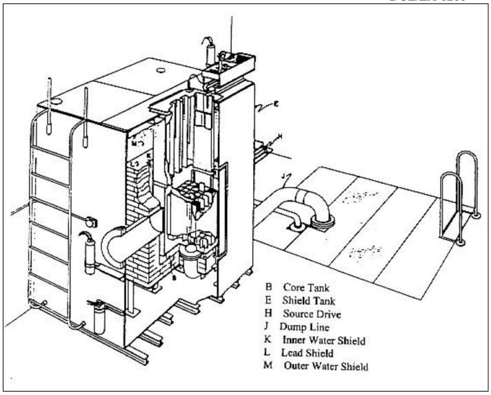
Figure 4 Isometric Cutaway of Argonne Thermal Source Reactor (Approximate Scale: 1" = 2.4')
