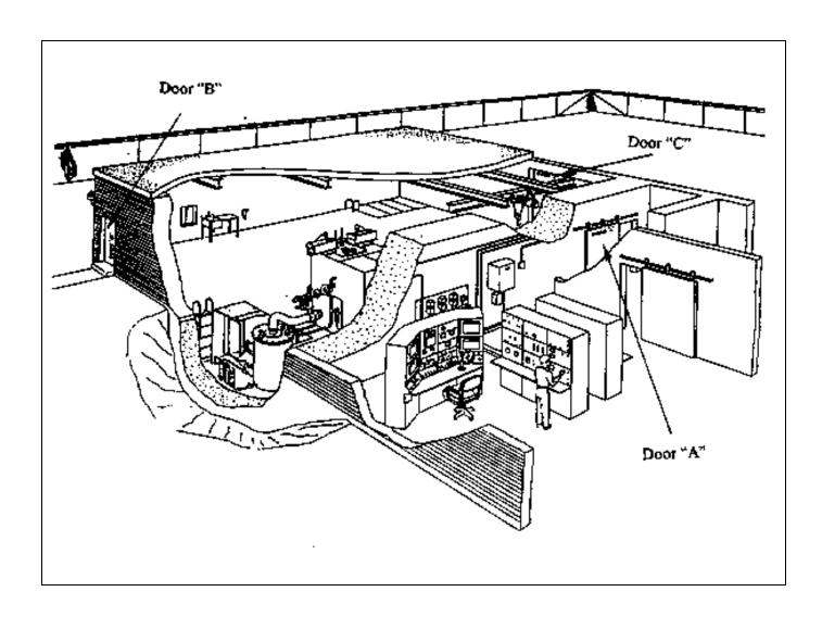
Figure 3 Argonne Thermal Source Reactor Facility Layout (Approximate Scale: 1" = 12')
