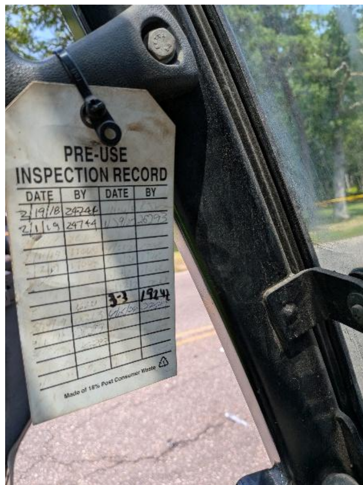
Figure 9: Forklift pre-use inspection tag after the accident on July 1, 2026.
