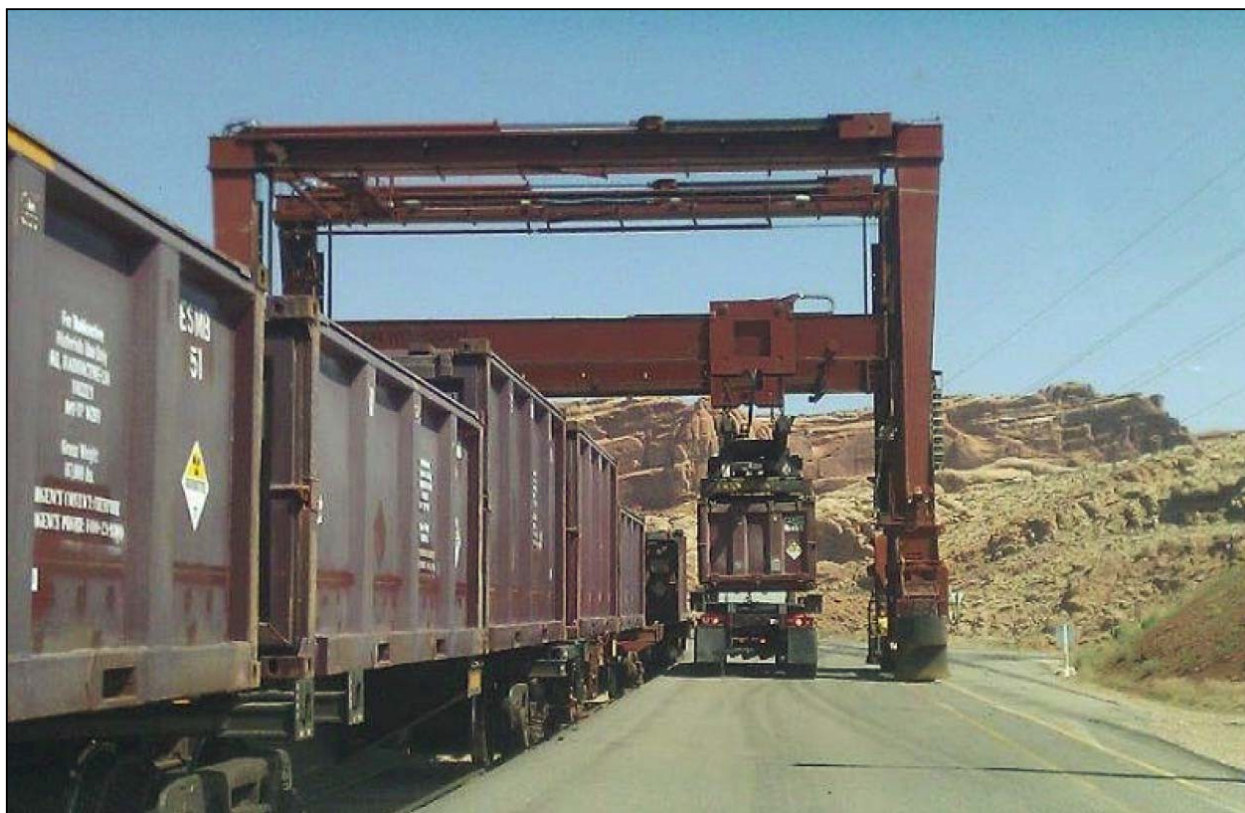
Figure 5. RRM Containers on Railcars
