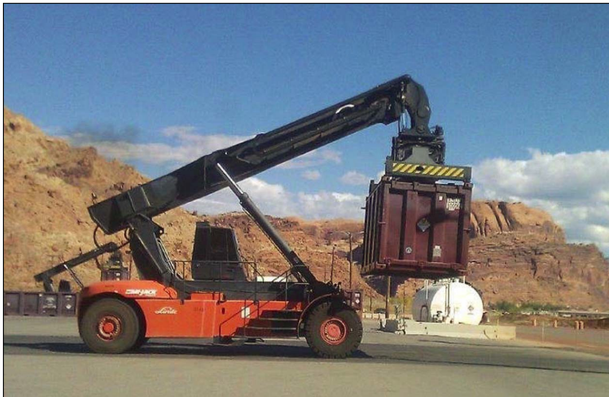
Figure 4. RRM Container Lifted by Reach Stacker
