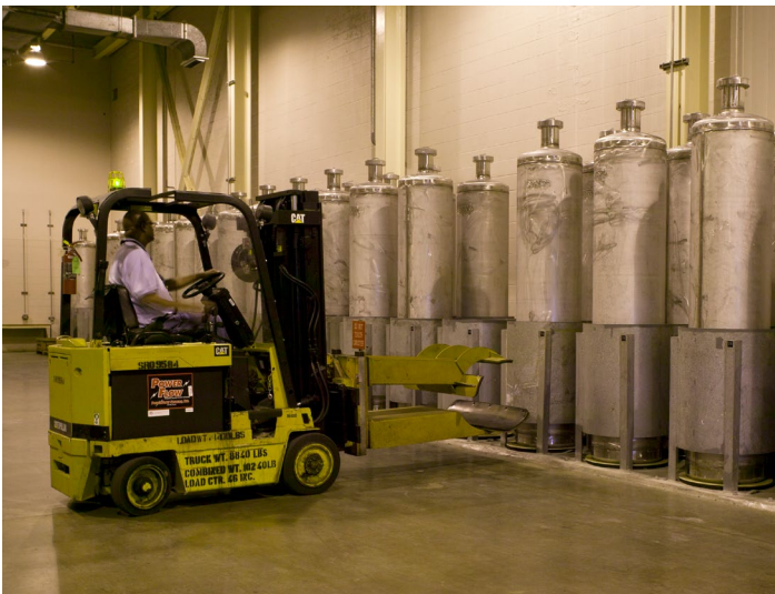
Workers use a special forklift to move an empty canister for its inspection at DWPF. The canister will be filled with vitrified high-level waste.
