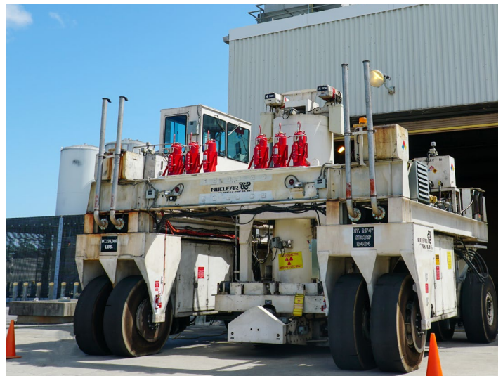
The Shielded Canister Transporter is used to move filled canisters to storage inside the Glass Waste Storage Buildings.
