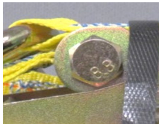
Ratchet strap with 8.8 marking and no manufacturer marking
