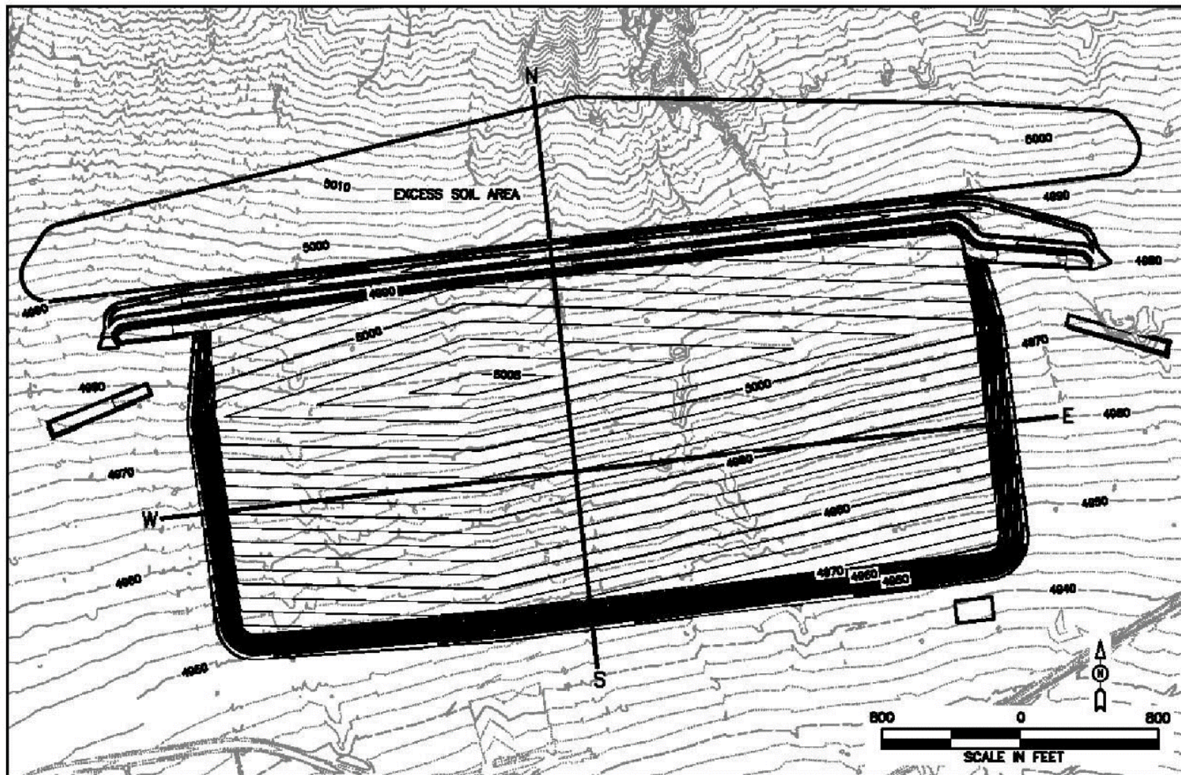
Figure 19. Disposal Cell Layout with Typical Cross-Section Locations
