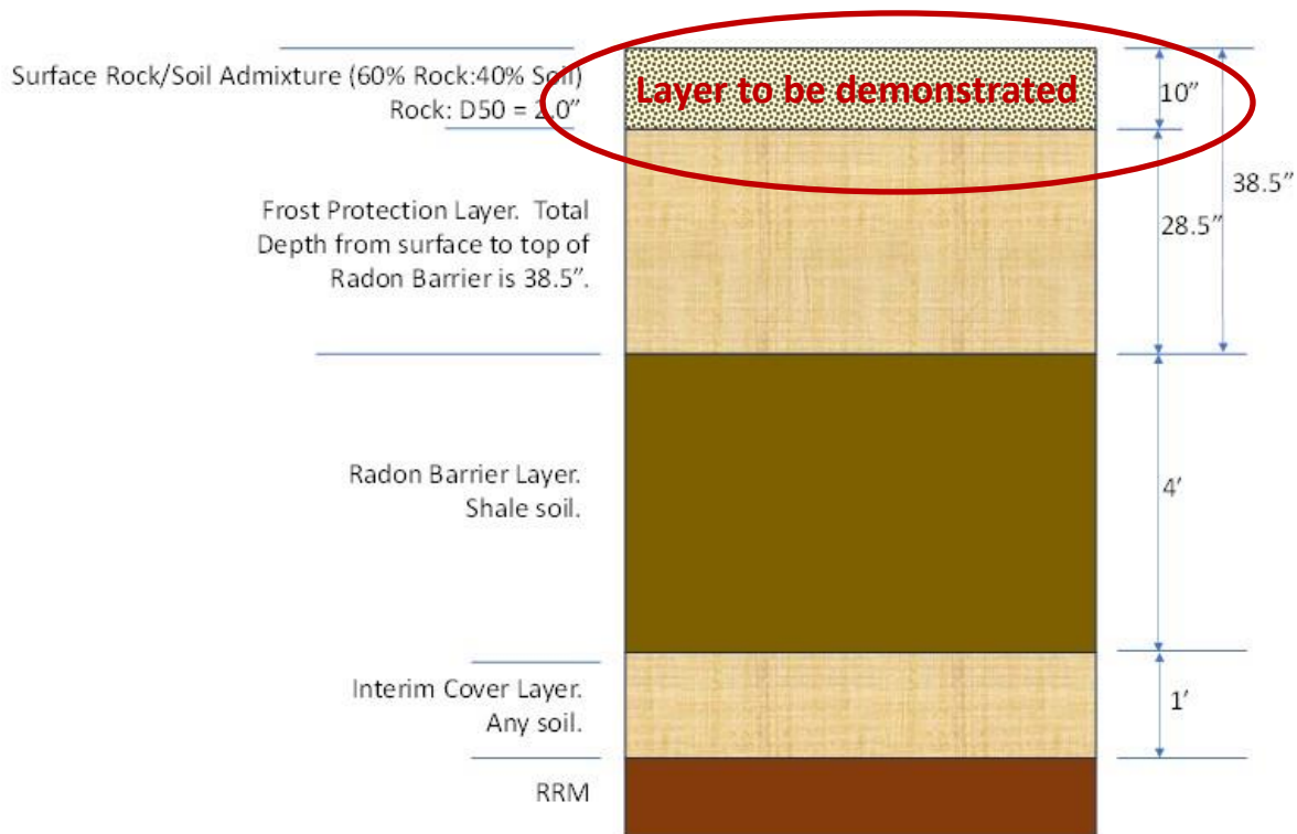
Figure 1. ET Cover Profile with Surface Admixture Layer
