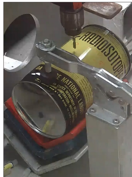
OREM crews use gloveboxes to vent canisters of legacy oxide waste generated from previous research and development activities at ORNL.
