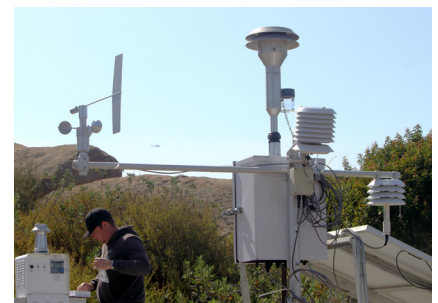
A DOE contractor changes out the filter in one of the perimeter air monitors during the Sandy Fire. Photo courtesy of Josh Mengers.
