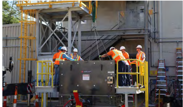
Teams move downblended U-233 material using an air pallet
