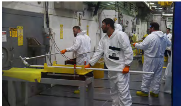
Employees load a canister of U-233 into a hot cell for processing
