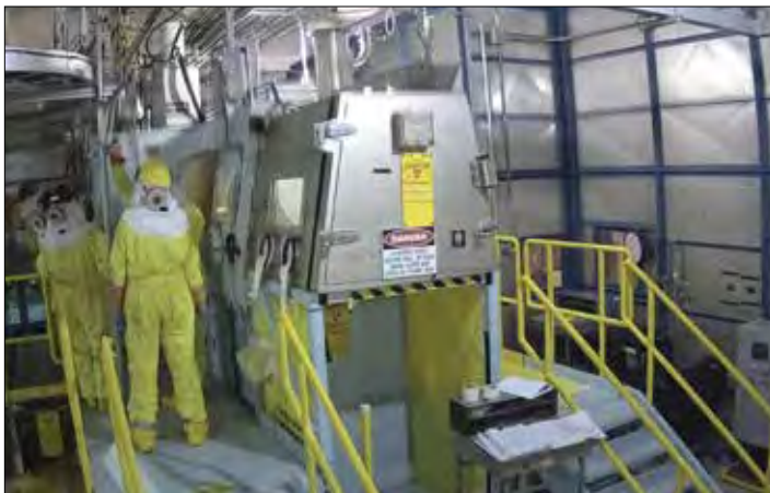
Transuranic Waste Processing Center workers safely replaced the facility's 900-pound waste-drum crusher, restoring the center's full waste processing capabilities for an ongoing cellulosic waste campaign.
