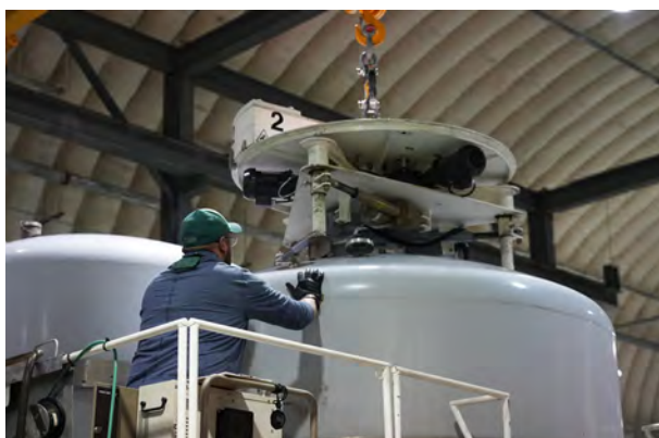
Workers load processed TRU waste into a shipping cask
