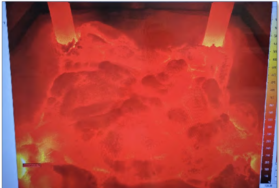
The GeoMelt technology heats the sodium shields to more than 2,700 degrees Fahrenheit, turning the reactive metal into a stable glass form for safe, permanent disposal through a process known as vitrification.
