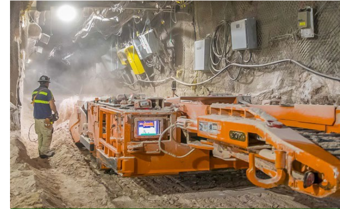
Crews use a machine called a continuous miner to level the floors, 2150 feet below the desert surface at the WIPP
