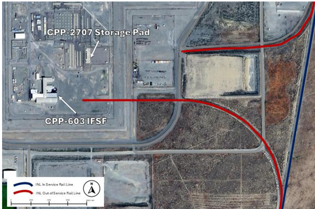
Figure 1-9. Idaho Nuclear Technology and Engineering Center rail access options (Idaho National Laboratory site).
