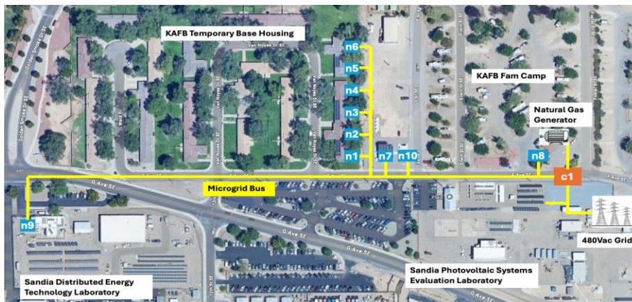
Figure 5. Layout of the Kirtland AFB microgrid. It is composed of load-serving nodes with nanoblocks (blue), a 750 V interconnection dc bus (yellow), and a central energy storage system (orange) with grid and backup NG generation.
