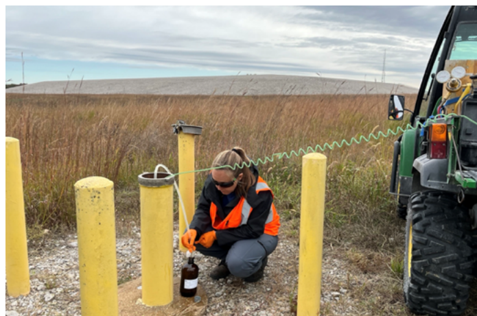
Groundwater samples are taken regularly and analyzed to confirm the cell is working as intended.
