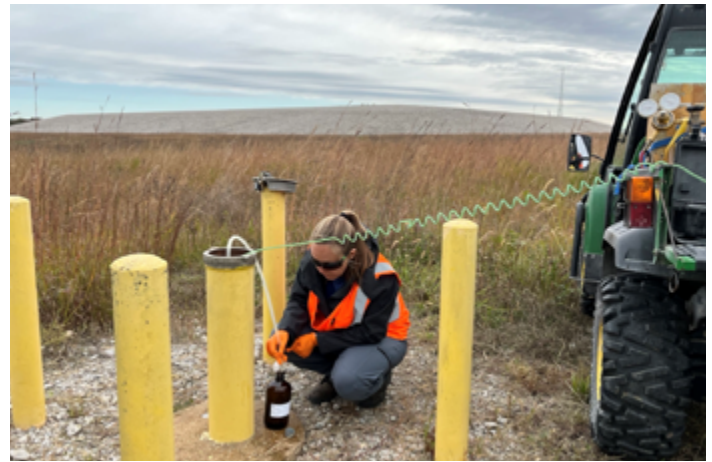
Groundwater samples are taken regularly and analyzed to confirm the cell is working as intended.
