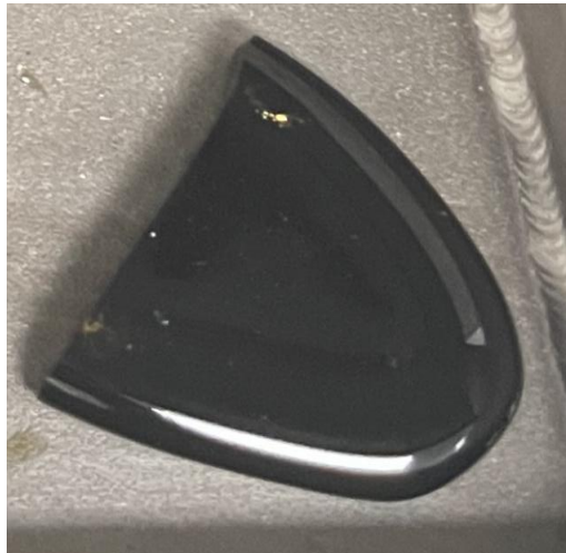
Figure C.34. Photograph of HAL24M2-04-1 glass after the third melt.
