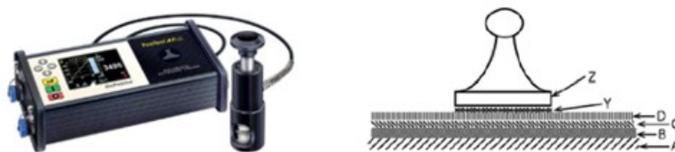
Figure 2. Pull tester instrument shown on left. Adhesion dolly fixture on right. Z is dolly fixture, Y is glue, D thru B are successive coating layers if more than one coat is applied, A is the adherends (in our case steel and cementitious grout).
