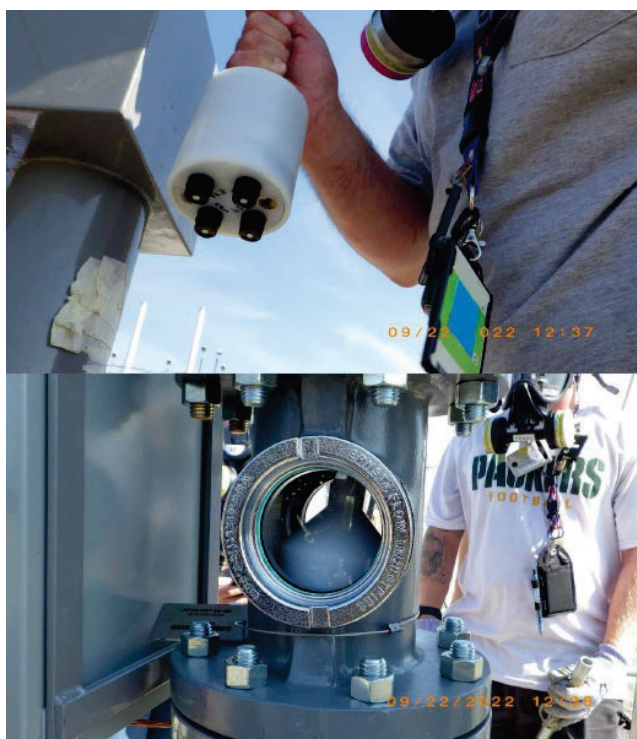
Figure 2-9. Four VLSJ Ag/AgCl reference electrodes mounted in RCMP probe head (top) and installation via riser in Tank 241-AP-106 (bottom) 21 .
