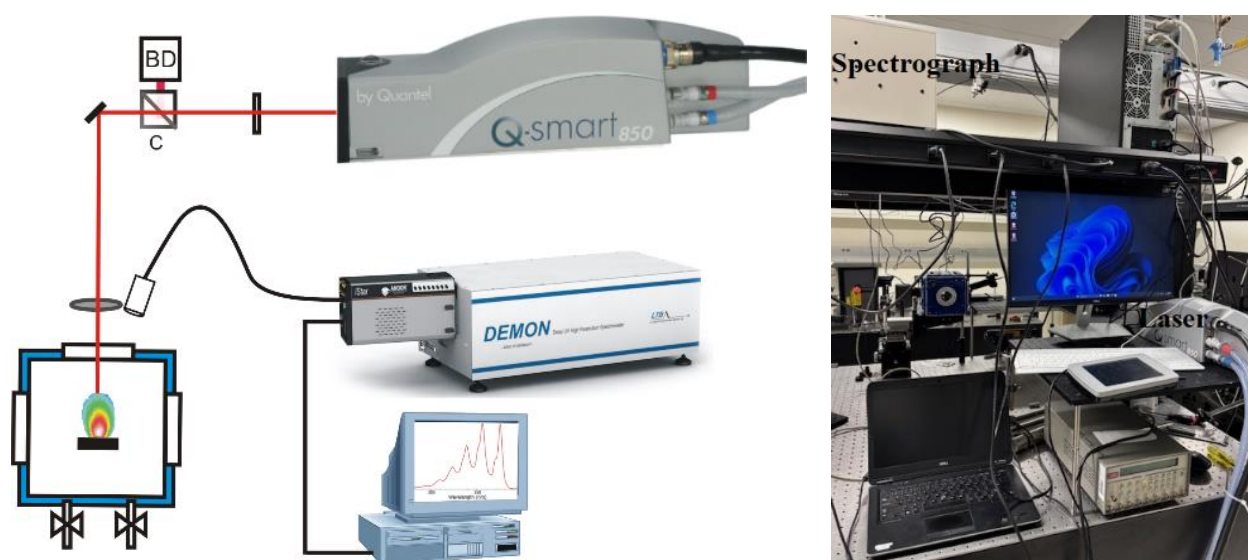
Figure 9. (left) Schematic of the LIBS set-up developed for slurry analysis. (right) photograph of the set up.
