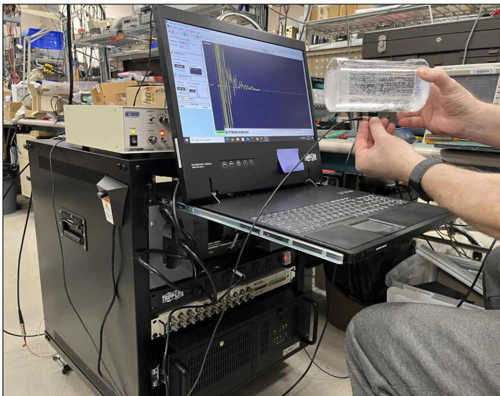
Figure 30. Photograph of a UPE transducer signals displayed on the UPE DAS during bench-scale functional testing in February 2025.
