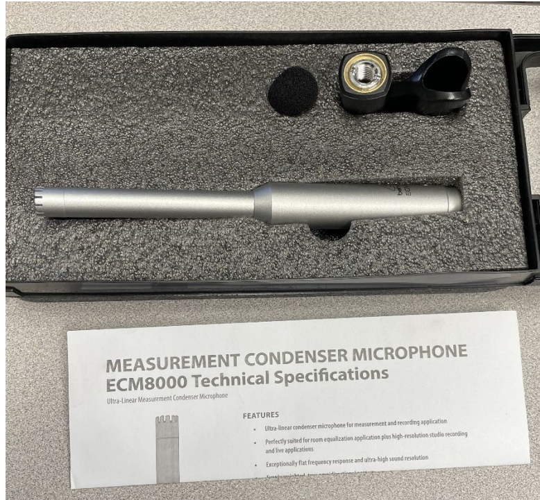
Figure 10 - Condenser microphone used to measure acoustic waveforms from the LIBS plasma formation.
