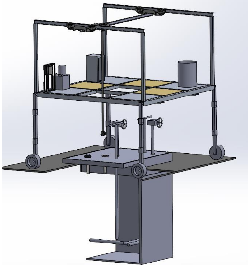
Figure 2. Adjustable full system support frame concept.
