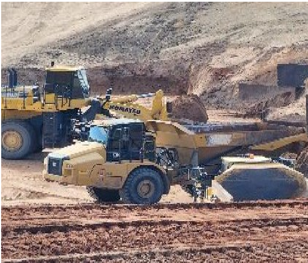
Photo 7. Loader Loading RRM into Haul Trucks. January 2025
