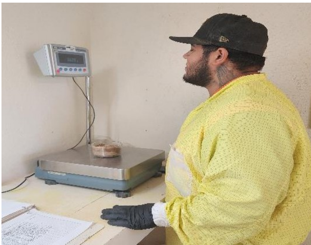
Photo 21. QC Weighing an RRM Moisture Sample in the Lab. August 2025
