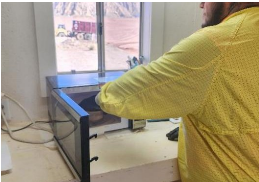
Photo 22. QC Drying an RRM Moisture Sample in the Lab. August 2025
