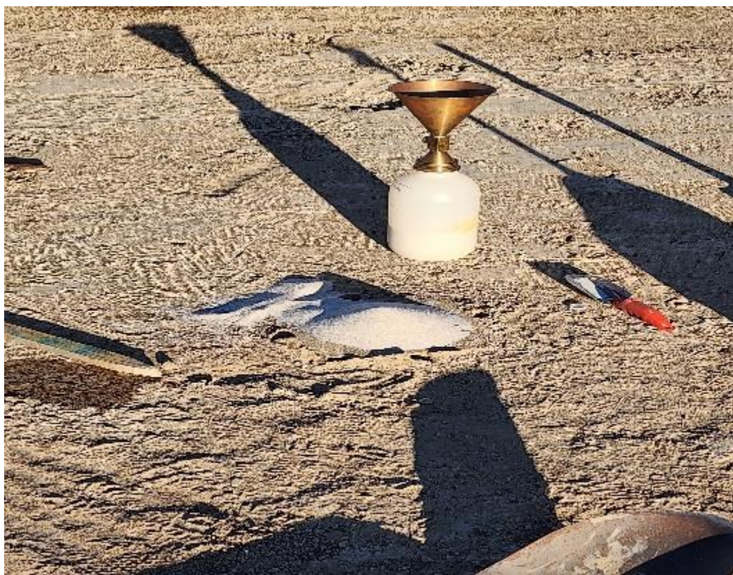
Photo 30. QC Finished a Sand Cone. September 2025
