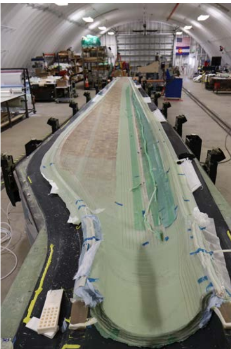
Figure 6 (left) and 7. Researchers at the National Renewable Energy Laboratory (NREL) construct a 13-m thermoplastic composite blade at NREL's Composites Manufacturing Education and Technology Facility. Photos by Ryan Beach, NREL
