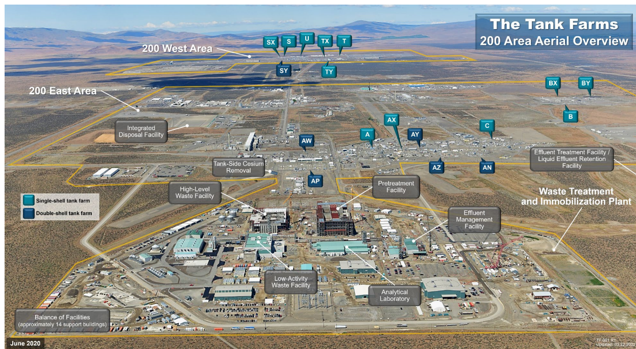
Figure 2-1 General Layout of the Hanford Tank Waste Treatment Complex
