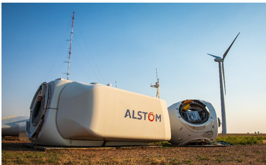
Figure 8. Decommissioned 3-MW GE/Alstom research wind turbine at NREL's Flatirons Campus. Photo by Werner Slocum, NREL 62412
