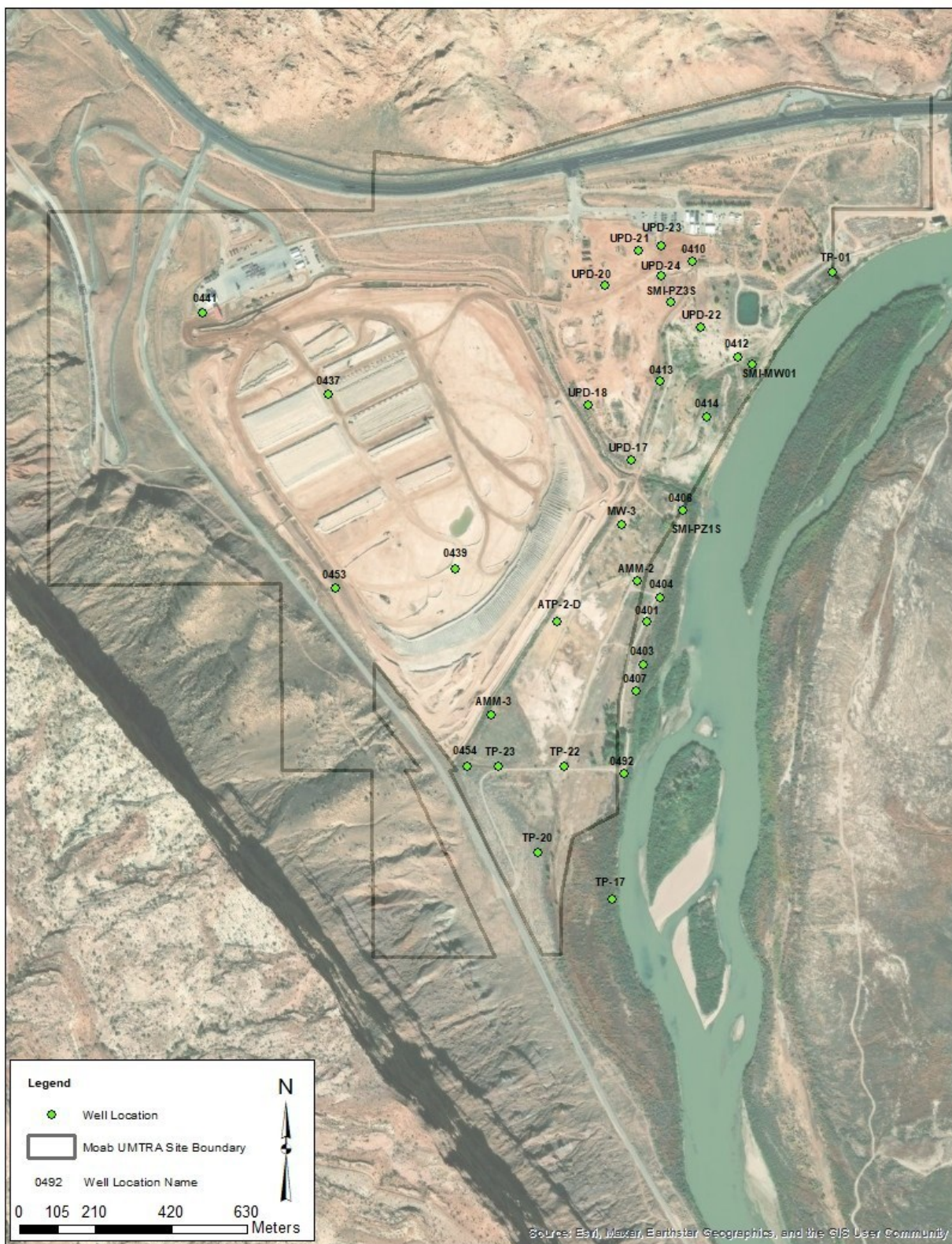
Figure 1. 2025 Site-wide Groundwater Sampling Locations
