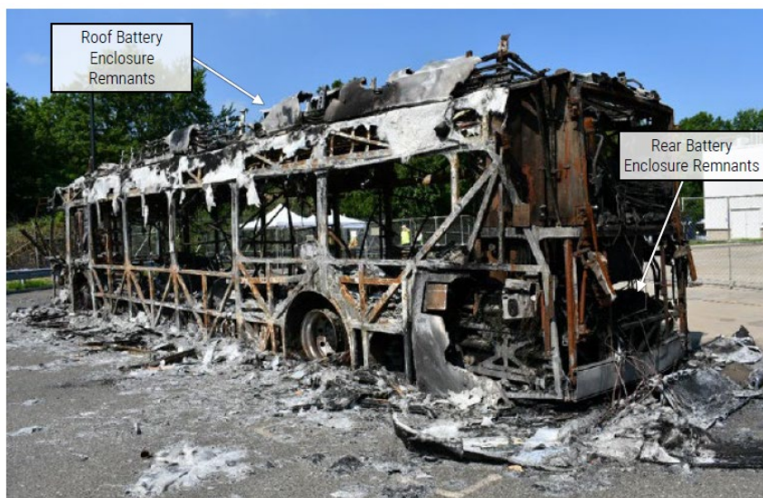
Figure 3: Fire on Battery Electric Transit Bus 5
