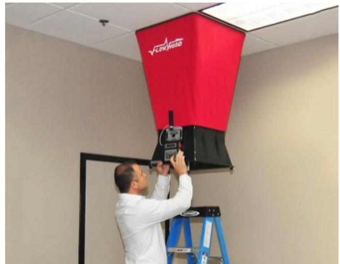
Figure 4 Specialist testing the flow rate of a supply vent to verify ventilation effectiveness. Source: Local Energy Audits.
