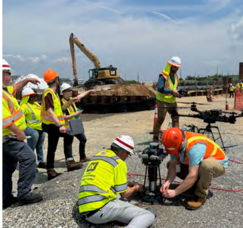
Members of USACE, the Ramboll Group, and Lawrence Berkeley National Laboratory prepare drone-mounted radiological screening equipment at the Deepwater, New Jersey, Site.
