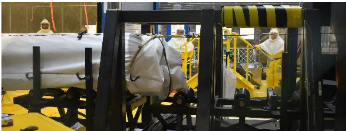
Moving the CMP into position for cutting with the shear
