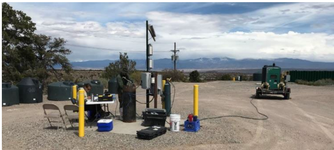
Typical setup for sample collection at a regional groundwater monitoring well
