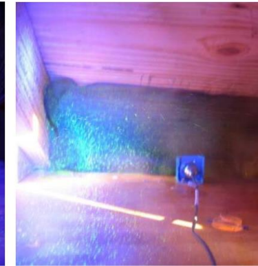
Wind Driven Rain Visualization with Fluorescent Tracer Dye ( Masters 2006 )
