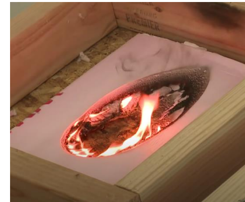
Example comparison between a vent with an intumescent coating and one that does not ( Ember Defense LLC, n.d. ) Dr. Energy Saver. (2013). Fire Testing Insulation Materials. YouTube Video .
