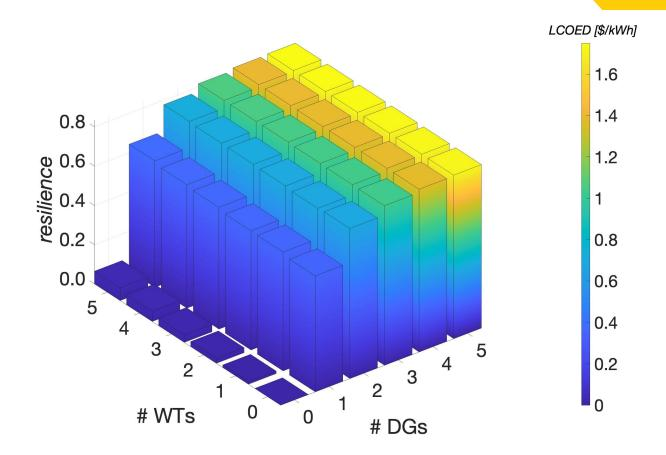
Relationship between resilience, number of wind turbines (WT), and number of diesel gensets (DG) at SNI. The color degrades from blue to yellow as *LCOED* increases.
