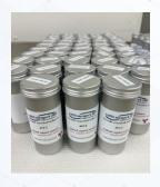
**HALEU Isotopic Reference Material:** ORNL has prepared a new 19.6 % <sup>235</sup>U enriched uranium isotope-amount ratio reference material for NBL Program Office. This new CRM was created as a gravimetric mixture of two high purity uranium metal
