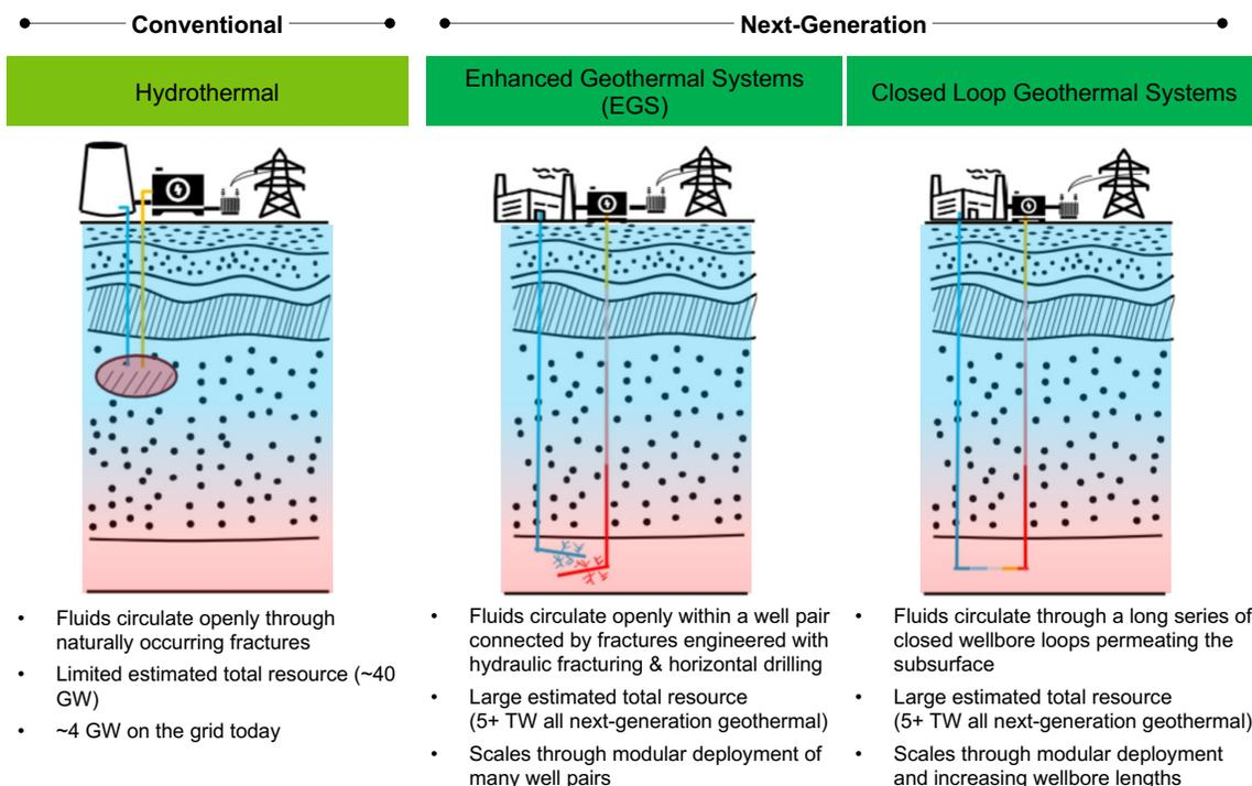
Figure 1: Geothermal technology overview across conventional (left) and next-generation (right) designs<sup>d</sup>
