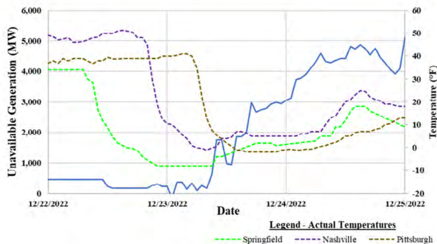
Figure 81: Unavailable Generation - Blackstart-Capable Generating Units, December 22 - 24, 2022
