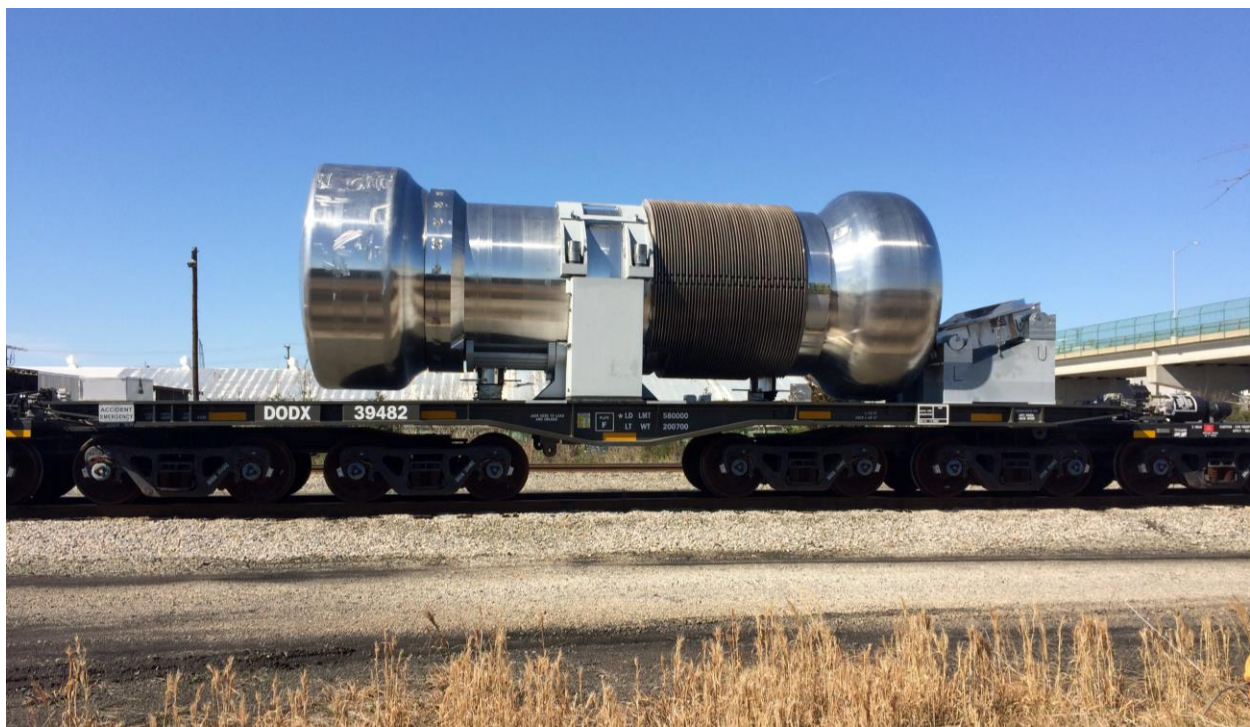
Robust shipping containers such as the M-290 are used to safely ship spent nuclear fuel.
