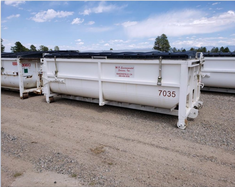
Twenty cubic yard roll-off with ~18 cubic meters of LLW soil debris generated from Middle DP Road Site Cleanup
