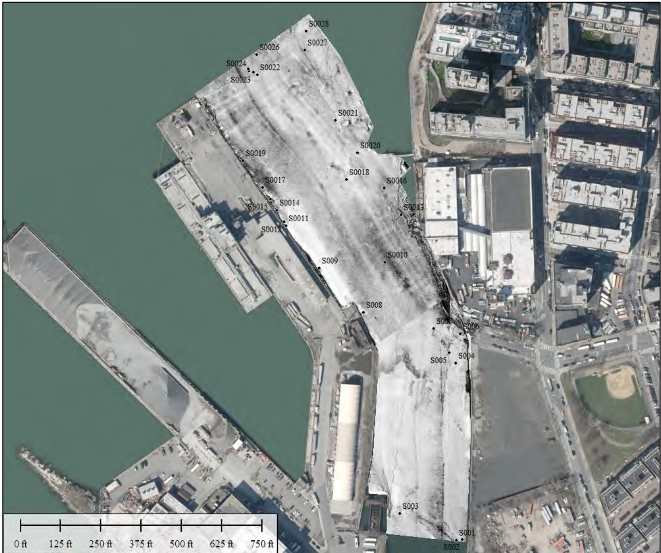
Figure 3. Side Scan Mosaic in Wallabout Channel (0.5ft resolution) with Contacts
