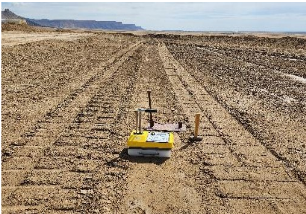
Photo 27. QC performing moisture/density test on Interim Cover July 2024
