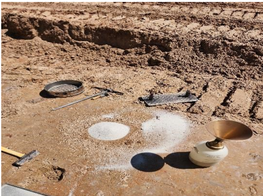
Photo 22. Sand cone test August 2024
