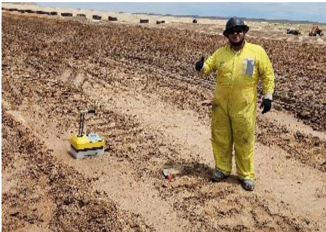
Photo 17. Moisture/density testing June 2024
