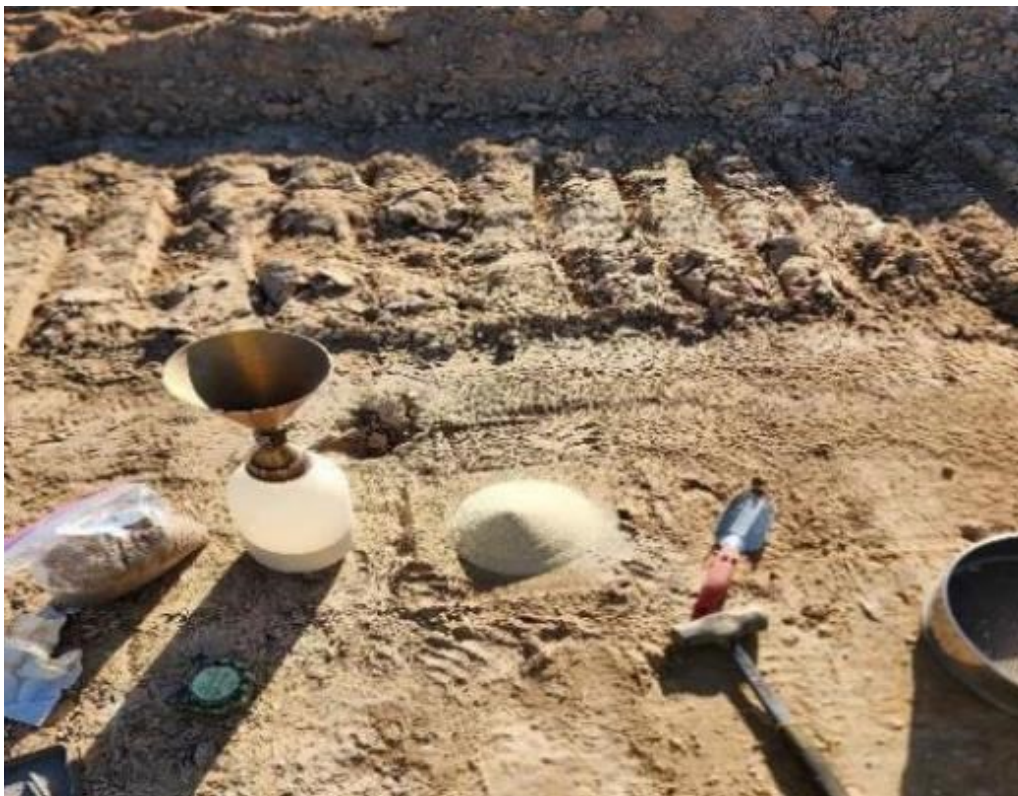
Photo 36. Finished sand cone on RRM lift September 2023
