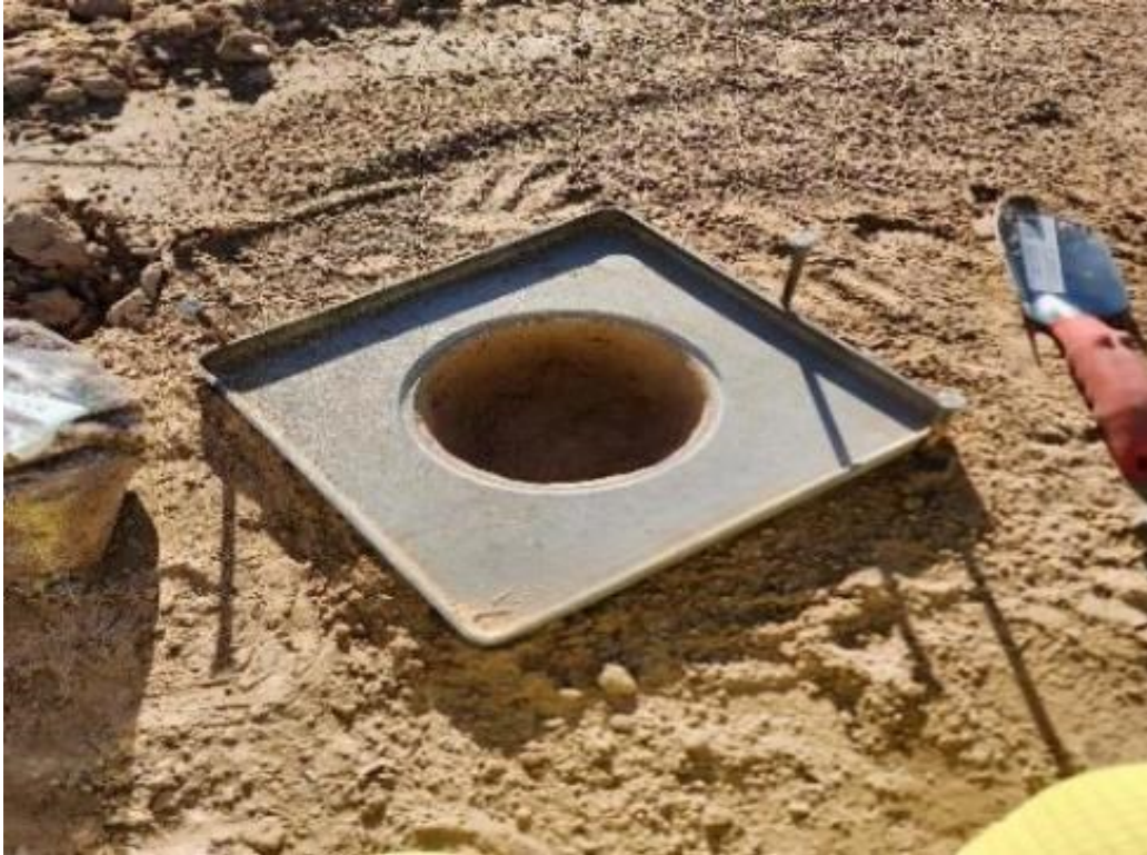
Photo 35. Hole for sand cone on RRM lift September 2023
