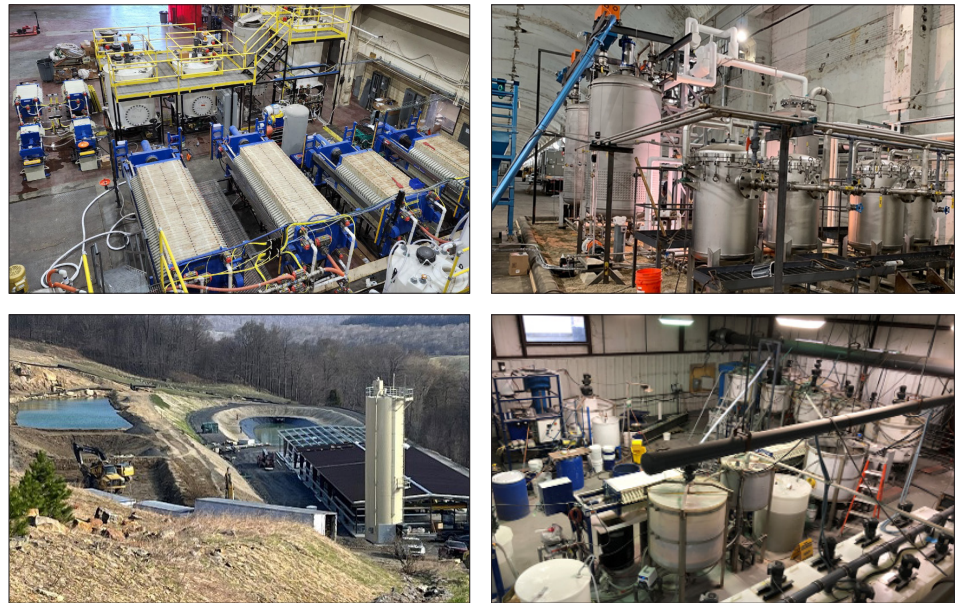
Figure 2. Small pilot facilities for processing rare earth elements from coal-based resources. Clockwise from top left lead performer and feedstock (University of North Dakota, lignite; Winner Water Services, coal ash; University of Kentucky, coal refuse and lignite; West Virginia University, acid mine drainage
