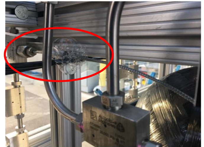
Small leak identified by a soap solution
