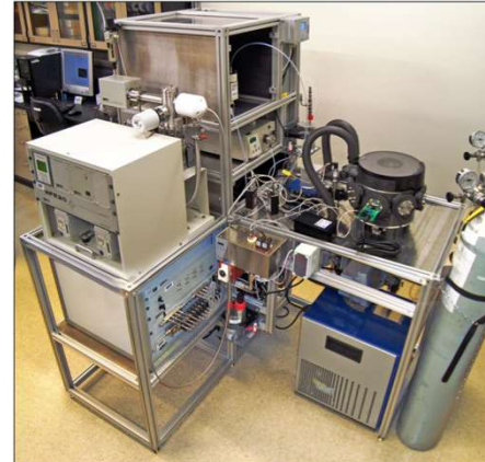
The SSTA Laboratory sensor test apparatus for safety and emissions sensor testing.
